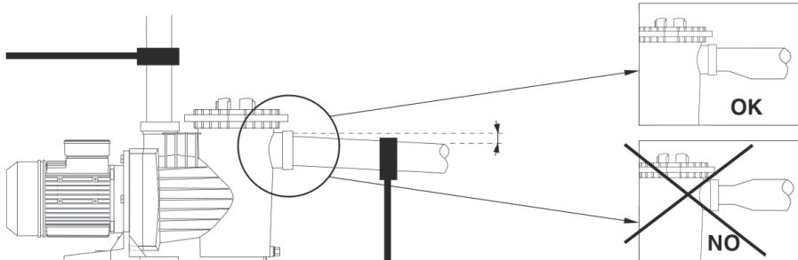
It is very important that both the suction and impulsion piping are independently supported and correctly fixed in place so that the pump does not have to support their weight nor the vibration produced by the water flow through them. In a situation where a long length of impulsion piping is used, we recommend the installation of a check valve to prevent the water hammer produced by the return of the water causing any damage when the pump stops.
