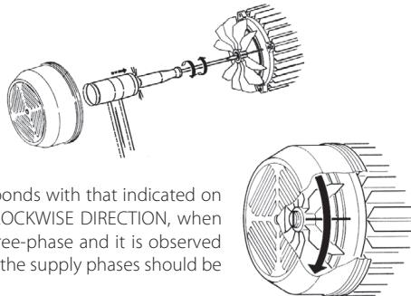
Check that the direction of motor rotation corresponds with that indicated on the specification plate (the fan should rotate in a **CLOCKWISE DIRECTION**, when viewed from the rear of the motor. If the motor is three-phase and it is observed that it is rotating in the opposite direction, then two of the supply phases should be inverted at the protection panel.
