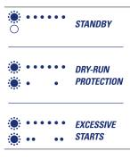
PRESFLO VARIO features 2 LED indicators to show the system's operating status and alerting to any issues through blinking patterns. A guide on the user interface helps to identify specific problems indicated by the LEDs.
